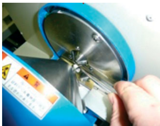
Figure 1. Introducing the sample into the DART mass spectrometer.
